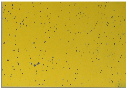
Plate 8. Water sensitive paper showing droplet stains for the blue nozzle, 2 m height and 2 bar water pressure treatment.
